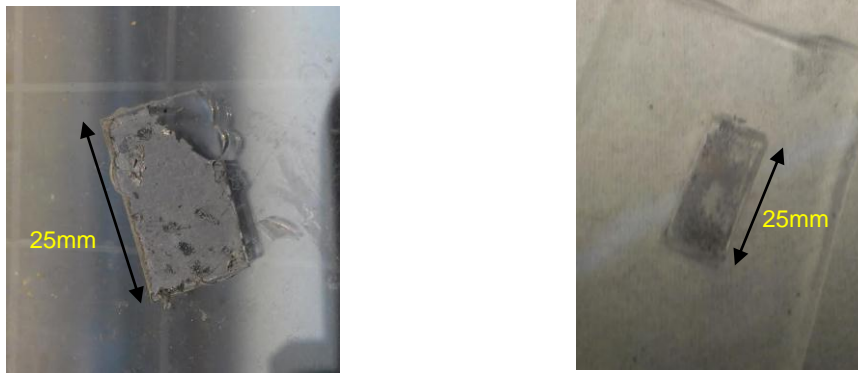
Figure 14: Result of a Wet Etch transfer and A Wet Peel Transfer.
